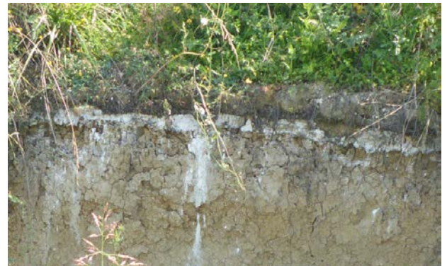
Figure 2: Soil horizon with a white layer of dumped HCH material (Photo by B.H.F. Boudewijn)
