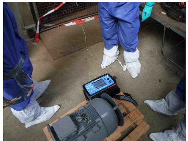
Figure 3 - Use of analyser to measure mercury concentration in air
